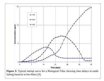
Instead of waiting up to forty days for the activation of the filter alive bacteria is proposed to be added to speed up the activation procedure. The expected levels of nutrients, as per some practical data that are collected from the author are presented in the following table 3.
